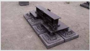
Proof tested 385kN Safe working load 295kN
